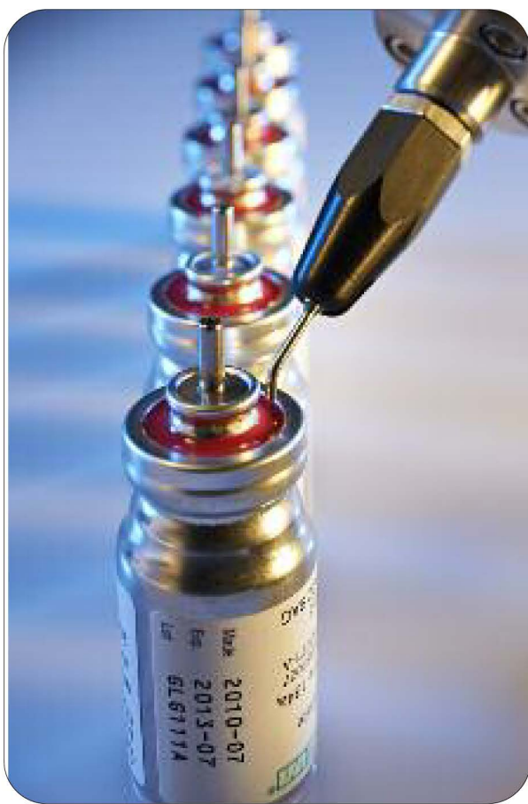
TS5440 - dispensing medical device adhesive
