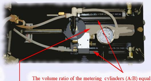
The mix/dispense valve assembly has an adjustable snuff-back feature and uses low cost static mixers
