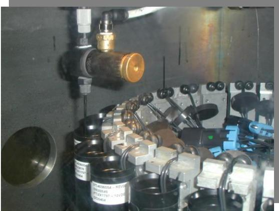
A vacuum chamber, capable of automatically processing 24 valves at varying vacuum levels was designed and integrated into metering system. The chamber was heated and incorporated a servo controlled rotary table and a vision system to detect the presence or misalignment of valves. If the system detected a misaligned or absent valve that shot would be aborted.
