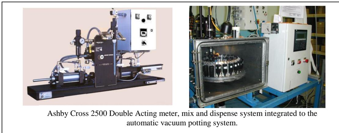
Once proportioned in the cylinders, the material moves to the heated mix/dispense head. The static mixer is housed in a shroud that penetrates the vacuum chamber. At this point the temperature is elevated to the final design point for pouring into the valve. By dispensing in a vacuum, elements within the valve, e.g., electric coil had no entrained air, providing for 100% penetration.
