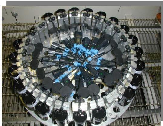
Encapsulated valves enter the conveyor oven for curing
