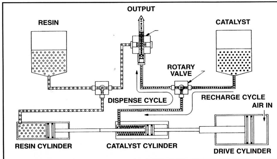
The Resin and Catalyst cylinders have a respective volume matching the volume mix ratio of the material to be processed. For instance, if the material has a 2:1 mix ratio (Resin:Catalyst) then the catalyst cylinder will have a volume equal to  $\frac{1}{2}$  the volume of the resin cylinder.
